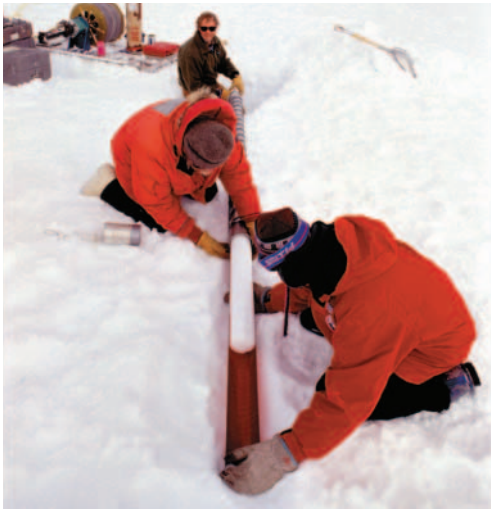
These scientists are removing an ice core from a thick ice sheet in Antarctica. Ice at the bottom end is oldest.
